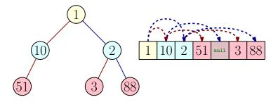
It gives fast access due to  $\mathcal{O}(1)$  lookup in arrays, but *potentially* wastes memory. Particularly advantageous for trees with full levels such as heaps.
