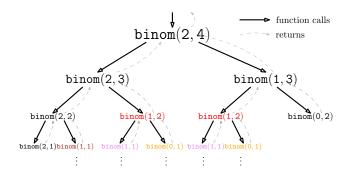
Dynamic programming or **memoization**<sup>7</sup> is essentially the technique that consists in avoiding these kind of redundant calls.
